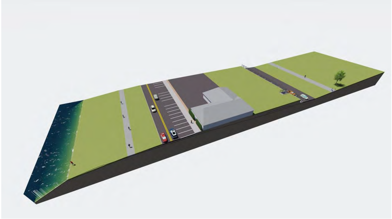
Typical Cross Section of downtown with fill from the river edge to Station Rd. at its current elevation
