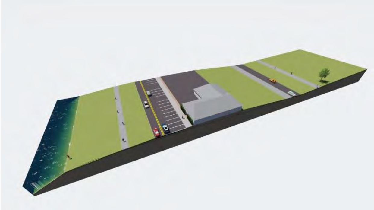
Cross Section of typical downtown with fill material elevating only Main Street Frontage
